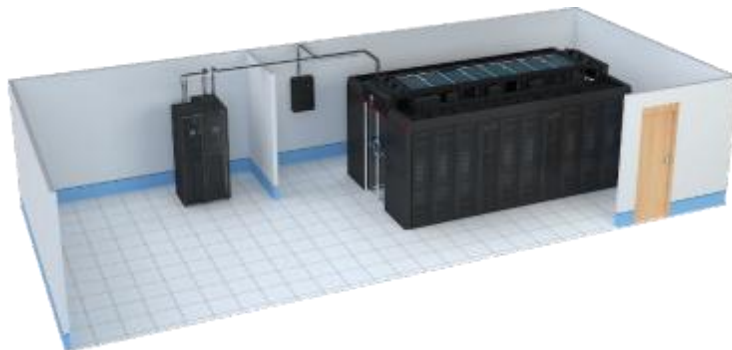
UPS Outside the Module(Smart Busway)
