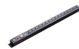
16 multiple outlets of 10A +1 double break switch + 1 overload protector+1 surge protector with 1 indicator
